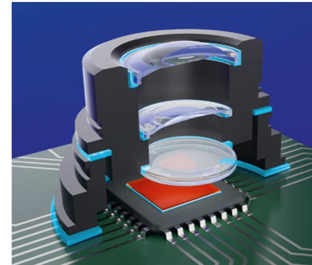
Our automotive-grade formulations feature a glass transition temperature designed specifically to lie outside the typical operating range, ensuring robust and proven long-term stability—even after 1,000 hours of testing.
