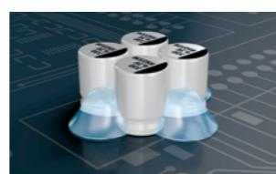
Frame-and-fill is a wet-on-wet process using two adhesives with different viscosities. A high-viscosity adhesive forms a perimeter frame, which is then filled with a low-viscosity adhesive. These systems are available as single-component, thermally curing adhesives (typically black) or transparent UV-curable adhesives for very short cycle times and are designed to minimize stress on component connections before and after curing.
